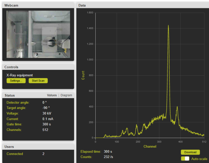
Figure 3: Screenshot of the calibration scan in the live experiment. The greatest peak originates from photons with an energy of 17.4 keV ( K_{\alpha} - decay of electrons in Molybdenum) and the second greatest peak originates from photons with an energy of 19.6 keV ( K_{\beta} - decay of electrons in Molybdenum).
